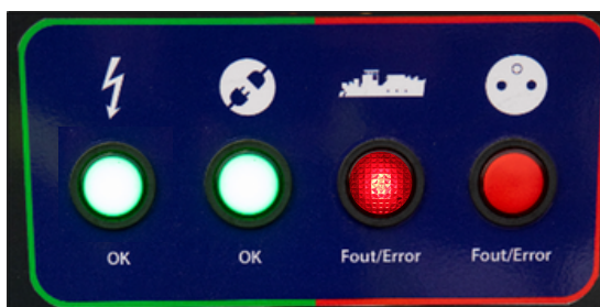
Boot fout LED knippert
