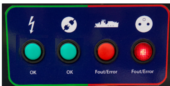
Stopcontact fout LED brandt vast
